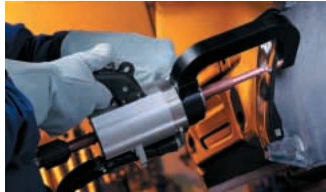
The C-Tong allows access to hard to reach areas.
