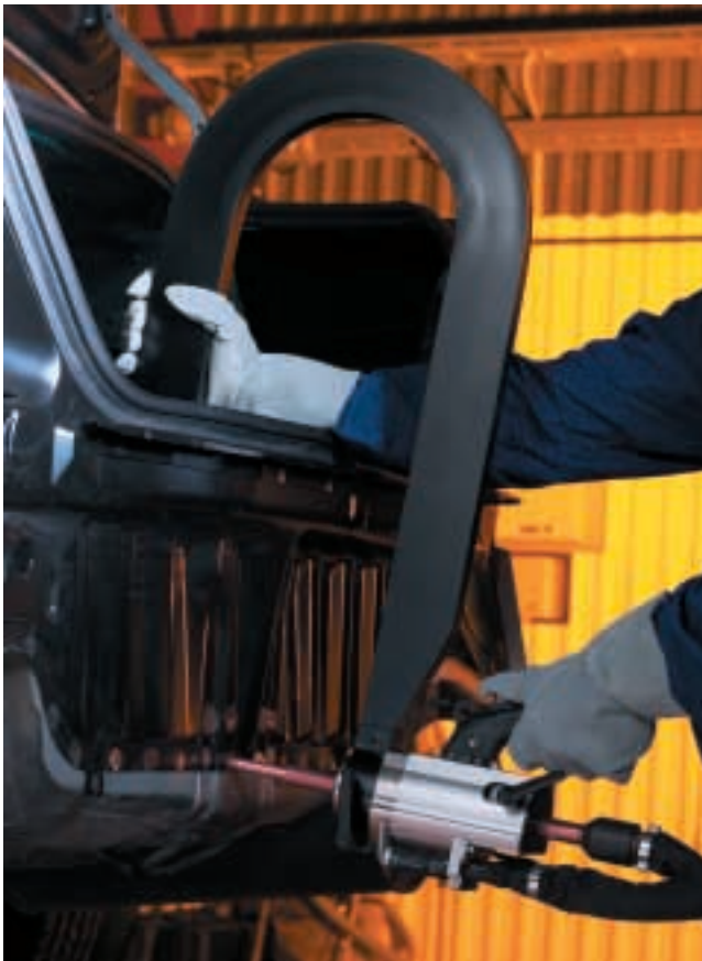
Extension yokes (optional) of different sizes allows access to hard to reach areas. Shown above, the 600 mm yoke.
